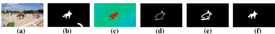
Fig. 2 Example of our motion based background suppression method. (a) Current frame \mathbf{I}_t . (b) Initial result \mathbf{IR}_t . (c) Optical flow \mathbf{F}_t . (d) Motion boundary probability map. (e) Dilated motion boundary map. (f) Purified result \mathbf{PR}_t
