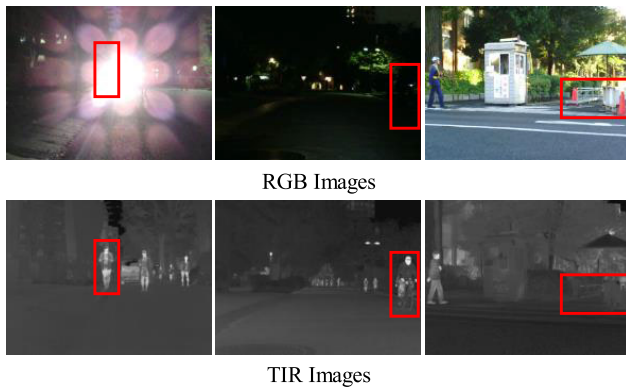
Fig. 2. Three typical scenes in RGB-T data. The first two scenes are nighttime scene with various unfavorable illumination conditions, and the last one is daytime scene. Please note the difference between the RGB image and the TIR image in the red box.
